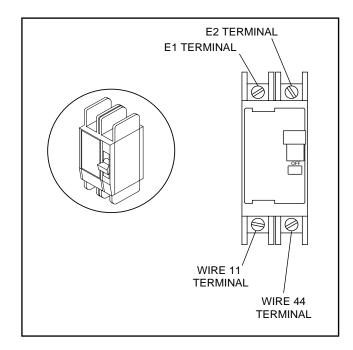
Figure 1. Generator Main Circuit Breaker Test Points
